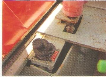
Parking brakes Pneumatically assisted fail safe brakes.
