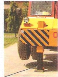
Stabilizers A special feature for maintaining stability while lifting load at maximum height.
