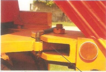
Front and Rear chassis joining Arrangement for achieving 40 deg. articulation on either side using heavy duty bearing for easy maneuverability and longer life.
