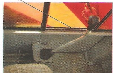
Gear Shift Gear shift through cables providing smooth gear shifting.
