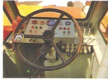
Power steering With double acting arms 40° articulation on either side.
