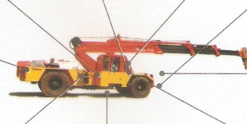
Power steering With double acting arms 40° articulation on either side.
