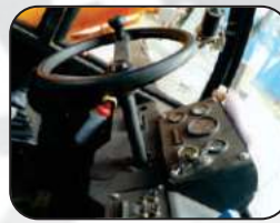
Power Steering With double acting arms 40° articulation on either side
